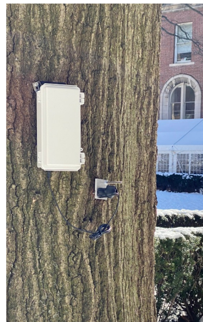
Data logger and dendrometer mounted on university tree.
